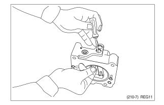
(8) Fit center plug (614) so that pin forcefitted in center plug (614) can be put into pin hole of lever (2).
