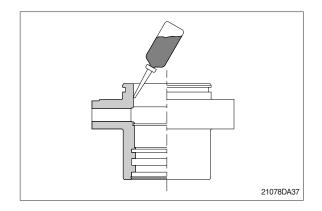
② Coat dust wiper (9) with grease and fit dust wiper (9) to the bottom of the hole of dust wiper.
