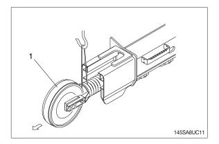
(3) Remove the bolts (2), washers (3) and separate ilder from recoil spring.
