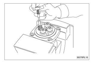
(3) Assemble O-ring (10) onto plug (8).
