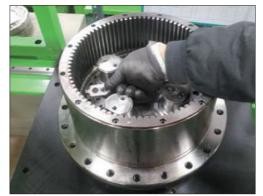
17) Disassemble nut ring (62) by using the jig.
