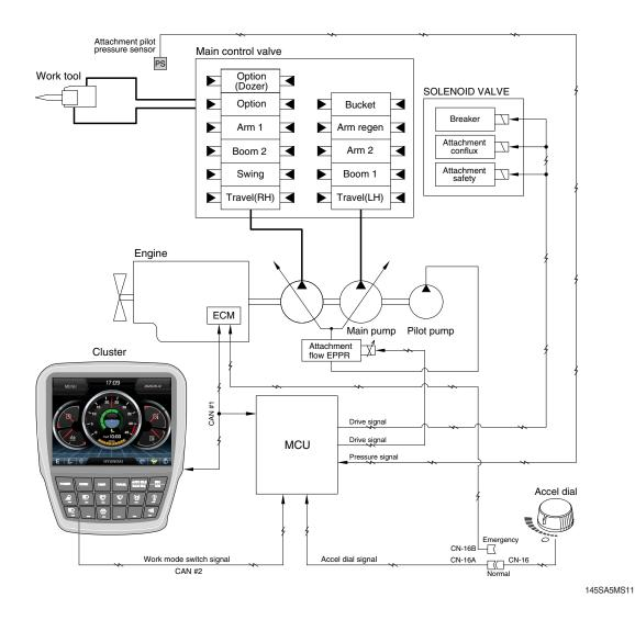
• The system is used to control the pump delivery flow according to set of the work tool on the cluster by the attachment flow EPPR valve.
