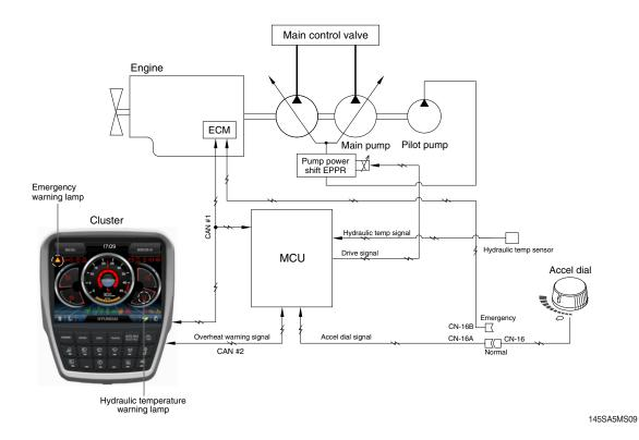
1. If the engine coolant temperature or the hydraulic oil temperature is overheated over set temperature, the warning lamp is ON and the pump input torque or the engine speed is reduced as below logic table.
