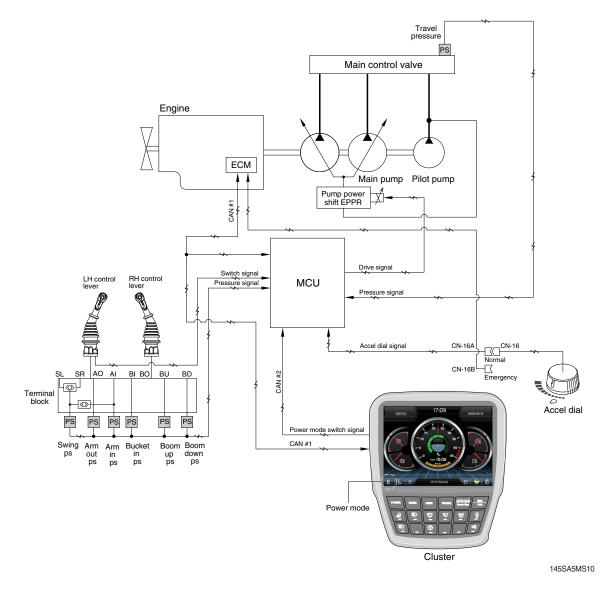
The new variable power control system makes constantly exact pump control through improvement variable engine speed control and response and optimization of control input sensor signal.
