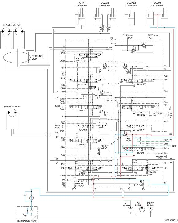
When the right control lever is pushed forward, the boom 1 spool in the main control valve is moved to the down position by the pilot oil pressure (Pb20) from the remote control valve.
