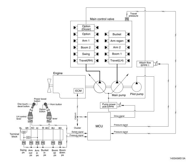
1. When the requirement of pump flow rate is low, IPC mode controls pump flow rate to improve fuel efficiency.
