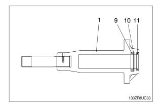
② Pour grease into body (1), then push in rod (12) by hand.
