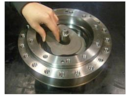
(7) Assemble spring (13) (9ea) and ball guide (14) in cylinder block (12) in that order.
