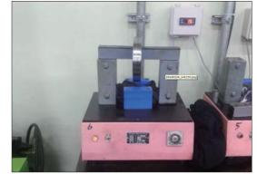
(19) Shrink fit taper roller bearing (3) on drive shaft, complete drive shaft sub assembly.
