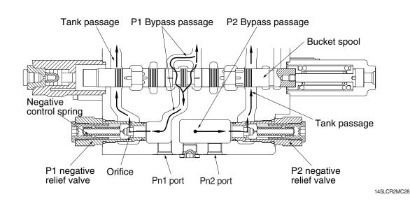
For the pump A1 the same negative control principle.
