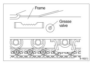
(2) Jack up the track link height enough to permit upper roller removal.
