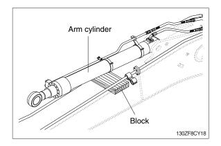
Remove bolt (2) and pull out pin (1).
