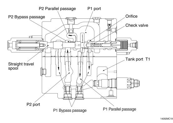
This function keeps straight travel in case of simultaneous operation of other actuators (boom, arm, bucket, swing) during a straight travel.
