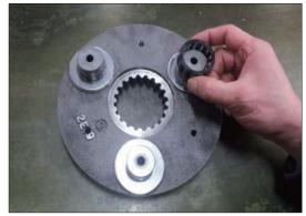
(9) Disassemble thrust washer No.1 (lower) (20).(3 pcs)
