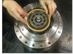
(11) Insert back-up ring & O-ring in parking piston.
