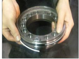
(21) From parking piston separate O-ring (20) and back-up ring (21).
