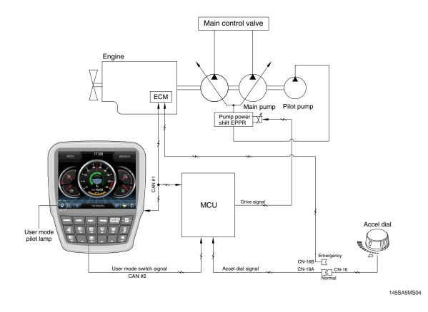
1) Engine speed, idle speed and pump power shift pressure can be adjusted and memorized in the U-mode.
