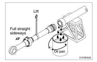
Note that the plated surface of rod assembly (2) is to be lifted. For this reason, do not use a wire sling and others that may damage it, but use a strong cloth belt or a rope.
