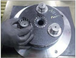
3) Assemble planetary gear No.1 (72) of which groove is faced downward. (3 places)
