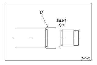
5 Fit piston assembly to rod assembly.  $\cdot$  Tightening torque : 150  $\pm$  15 kgf  $\cdot$  m
